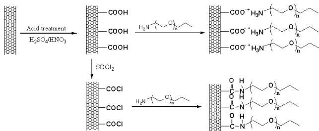
**Figure 1.** Reaction scheme of MWCNT/PEO-NH<sub>2</sub> complex through ionic and covalent bond.
