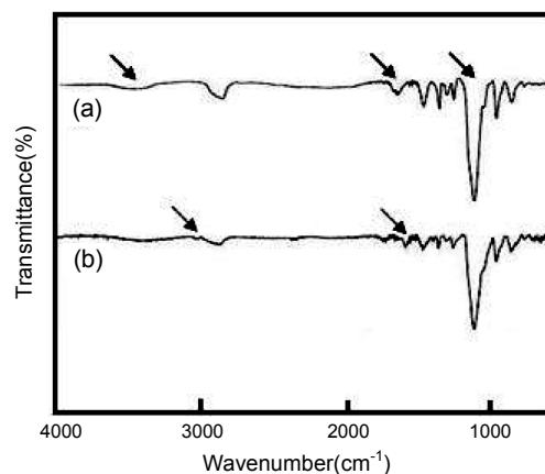
**Figure 4.** FTIR spectra : (a) PEO-NH<sub>2</sub>; (b) MWCNT-COOH/PEO-NH<sub>2</sub>.
