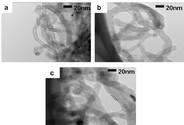
**Figure 6.** TEM images of (a) P-MWCNT; (b) MWCNT-COOH; (c) MWCNT-COOH/PEO-NH<sub>2</sub>.
