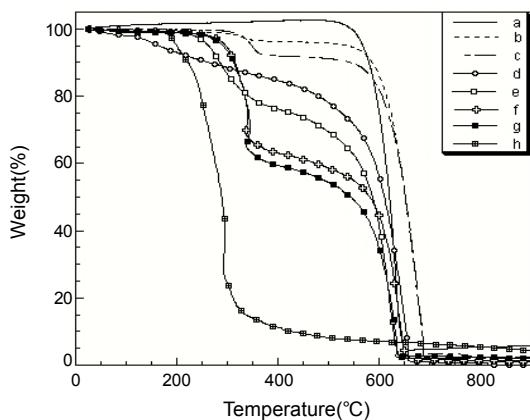
**Figure 3.** TGA thermograms of MWCNT/PEO complexes: (a) P-MWCNT; (b) P-MWCNT/PEO-CH<sub>3</sub>; (c) P-MWCNT/PEO-NH<sub>2</sub>; (d) MWCNT-COCl; (e) MWCNT-COCl/PEO-CH<sub>3</sub>; (f) MWCNT-COOH/PEO-NH<sub>2</sub>; (g) MWCNT-COCl/PEO-NH<sub>2</sub>; (h) PEO-NH<sub>2</sub>.
