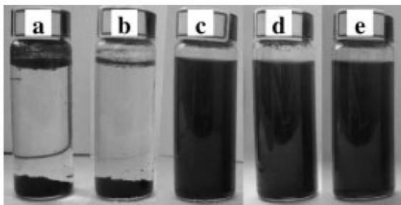
**Figure 2.** Dispersion of MWCNT and MWCNT/PEO complexes in water: (a) P-MWCNT; (b) MWCNT-COCl; (c) MWCNT-COCl-PEO-NH<sub>2</sub>; (d) MWCNT-COOH; (e) MWCNT-COOH/PEO-NH<sub>2</sub>.
