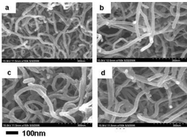
**Figure 5.** SEM images of (a) P-MWCNT; (b) MWCNT-COCl/PEO-CH<sub>3</sub>; (c) MWCNT-COCl/PEO-NH<sub>2</sub>; (d) MWCNT-COOH/PEO-NH<sub>2</sub>.
