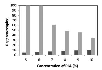
Figure 7. Effect of PLA concentration on s-PLA formation using sc-DME (250 bar, 70 °C, 1.5 h). The short black bars represent the total homopolymer (PDLA, PLLA) to total DME concentrations (%w/w) and the long grey bars represent the degree of stereocomplexation (%).
