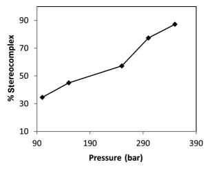
Figure 3. Effect of pressure on s-PLA formation using sc-DME (65  $^{\circ}$ C, 2 h).
