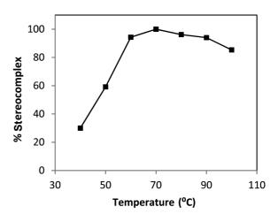
**Figure 4.** Effect of temperature on s-PLA formation using sc-DME (250 bar, 2 h).
