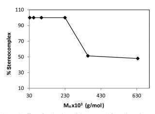
**Figure 6.** Effect of molecular weight on s-PLA formation using sc-DME (250 bar, 70 °C, 1.5 h).
