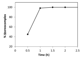
**Figure 5.** Effect of time on s-PLA formation using sc-DME (70  $^{\circ}$ C, 250 bar).
