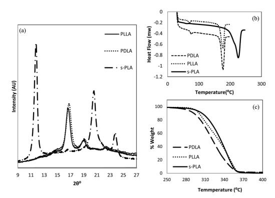
Figure 2. Comparison of PLLA, PDLA and s-PLA by (a) XRD; (b) DSC; (c) TGA analyses.
