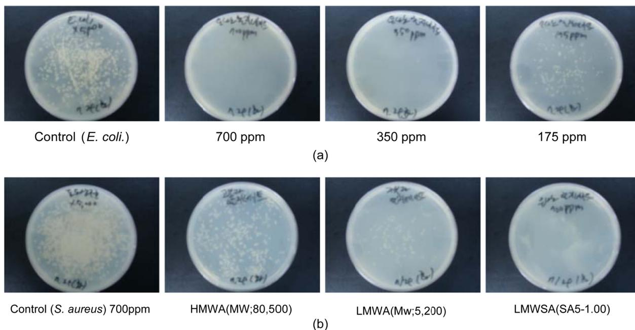
**Figure 4.** MIC of (a) LMWSA (SA5-1.00); (b) comparison of antibacterial properties of HMWA, LMWA, LMWSA at 700 ppm.
