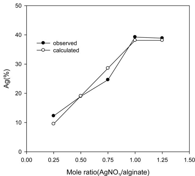
**Figure 1.** Ag content% vs. feed ratio in the LMWSA ( $M_w=5200$ ).
