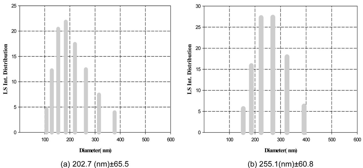
**Figure 2.** Particle size distribution of (a) LMWSA ( $M_w=5200$ ); (b) silver alginate (SA-5-0.50).
