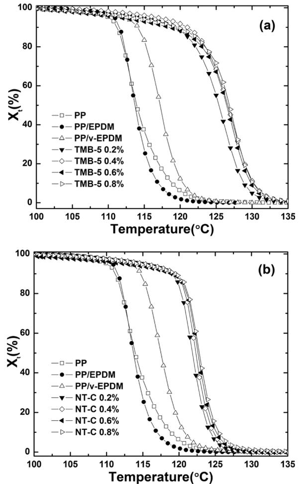
**Figure 4.** Evolution of relative degree of crystallinity ( $X_t$ ) as a function of crystallization temperature for various composites with different  $\beta$ -NAs: (a) TMB-5; (b) NT-C.
