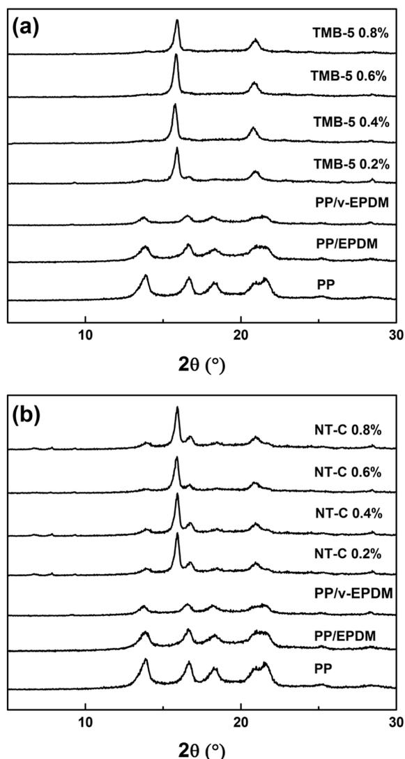
**Figure 2.** X-ray diffraction curves for various composites with different  $\beta$ -NAs: (a) TMB-5; (b) NT-C.
