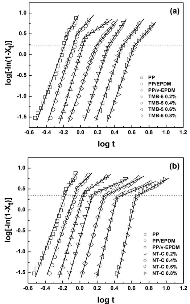
**Figure 3.** Plots of  $\log[-\ln(1-X_t)]$  versus  $\log t$  for various composites with different  $\beta$ -NAs: (a) TMB-5; (b) NT-C.
