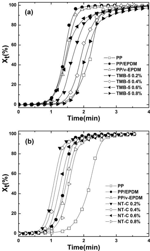
**Figure 5.** Evolution of relative degree of crystallinity ( $X_t$ ) as a function of crystallization time ( $t$ ) for various composites with different  $\beta$ -NAs: (a) TMB-5; (b) NT-C.
