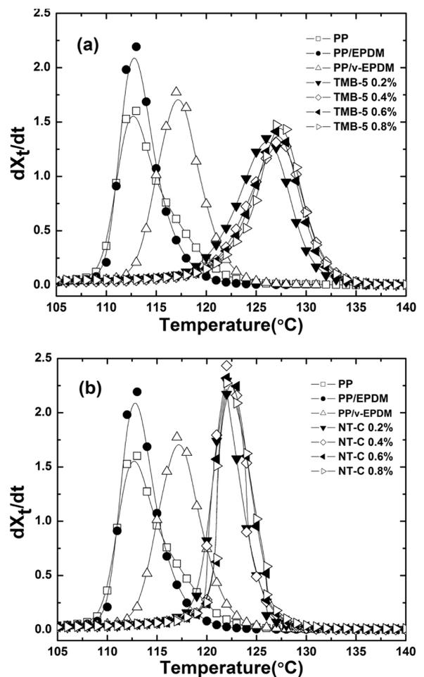
**Figure 6.** Variation of relative crystallization rate ( $dX_t/dt$ ) as a function of crystallization temperature for various composites with different  $\beta$ -NAs: (a) TMB-5; (b) NT-C.
