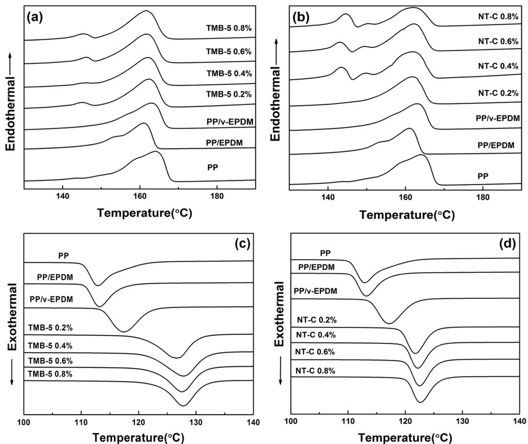
**Figure 1.** DSC heating and cooling thermograms for various composites with different  $\beta$ -NAs: (a) TMB-5 at heating; (b) NT-C at heating; (c) TMB-5 at cooling; (d) NT-C at cooling.
