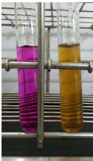
**Figure 2.** Images of a 0.02 M  $\text{KMnO}_4$  solution before (pink, left) and after (brown, right) added with 0.01 M EADA solution.
