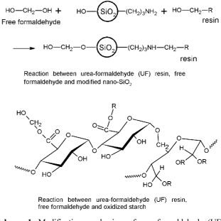
Scheme 1. Modification mechanism of urea-formaldehyde (UF) resin.
