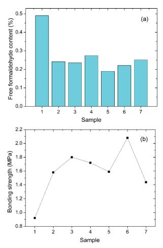
Figure 4. Free formaldehyde content (a); bonding strength (b) of sample  $1 \sim$  sample 7.
