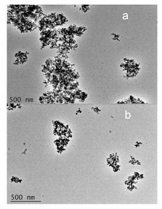
Figure 2. TEM microphotographs of pure nano-SiO $_2$  (a); modified nano-SiO $_2$  (b).
