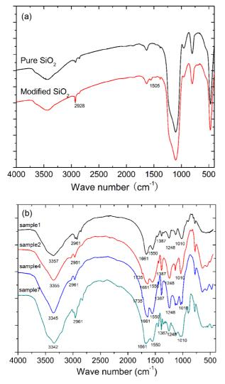
**Figure 3.** FTIR spectra of nano-SiO<sub>2</sub> (a); urea-formaldehyde (UF) resins (b).
