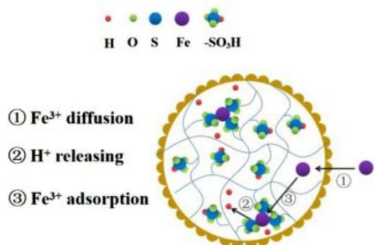
**Figure 6.** Process of Fe(III) adsorption with strong acid cation resin.
