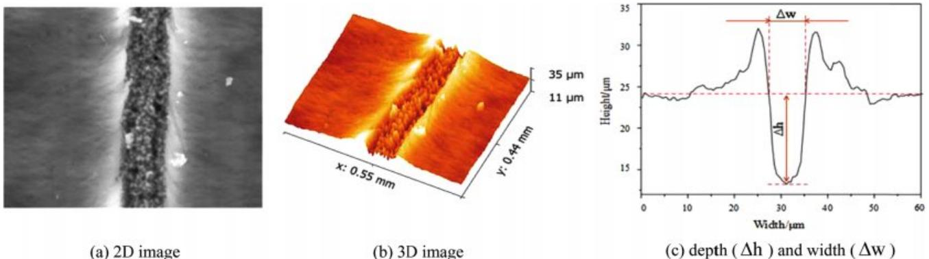
**Figure 10.** Scratch morphology of different materials.
