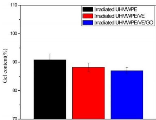
**Figure 7.** Gel content of different materials.
