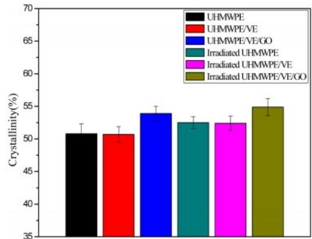
**Figure 6.** Crystallinity of different materials.
