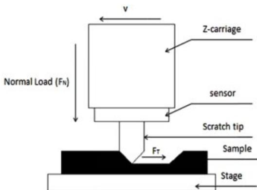
Figure 2. Diagrammatic sketch of scratch test.
