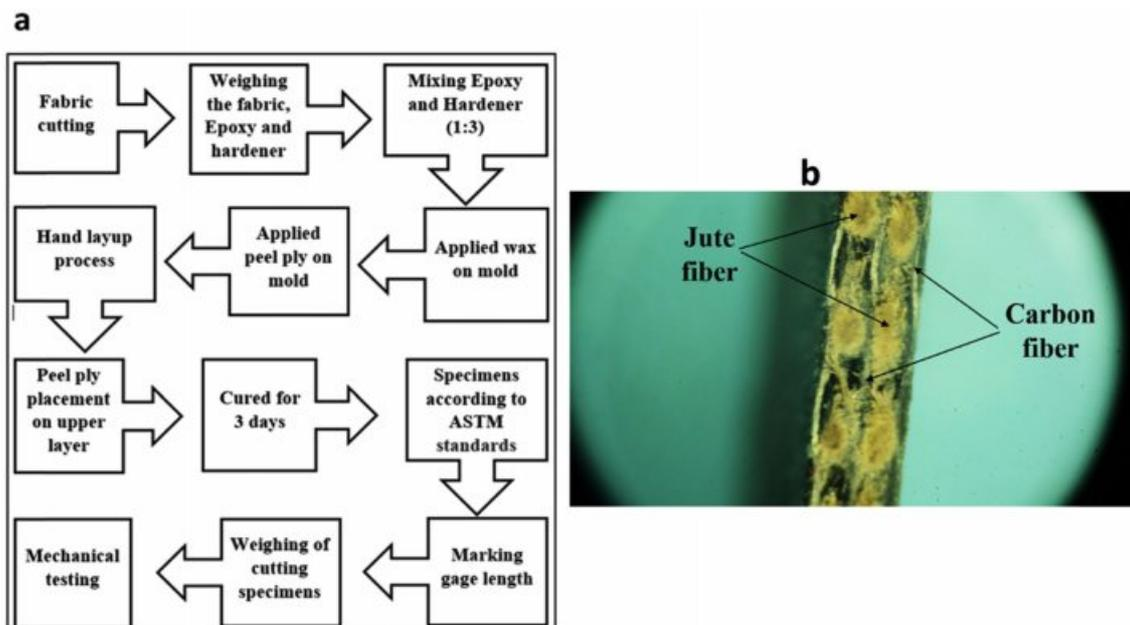
**Figure 1.** (a) Schematic plots of molding process for specimens; (b) stacking sequence of fibers.
