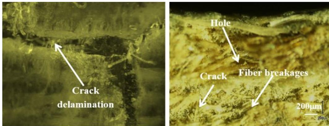
**Figure 7.** Damage pattern of samples under drop weight impact test.
