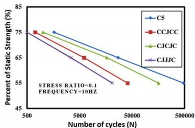
**Figure 3.** S-N curves at different loading condition in log linear cycles (N).
