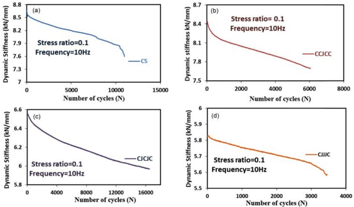
**Figure 4.** Stiffness degradation vs number of cycles to failures: (a) C5; (b) CCJCC; (c) CJCJC; (d) CJJC.
