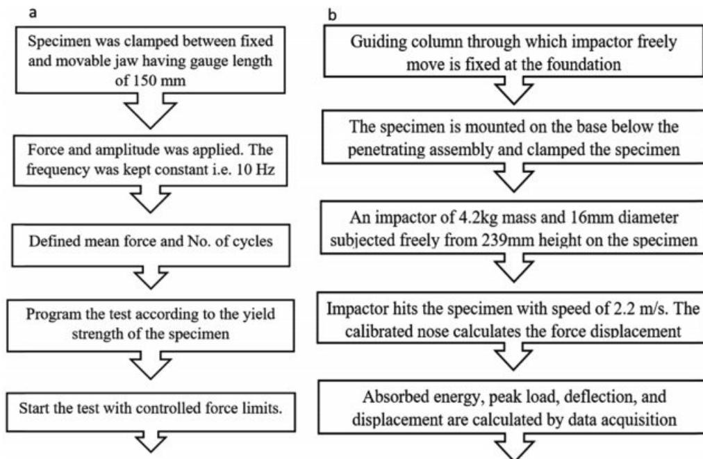
**Figure 2.** (a) Schematic representation of fatigue test performed on Zwick/Roell Z100 machine; (b) schematic representation of drop weight impact testing.
