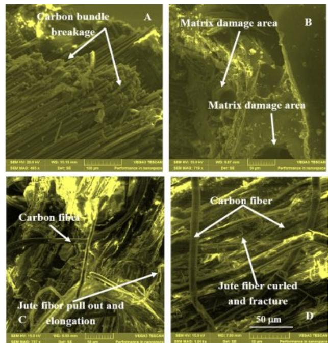
**Figure 5.** (a) SEM images of the CFRPs fractured under fatigue loading; (b) epoxy cracks after fatigue loading; (c) and (d) jute fiber pull-out and fiber breakage.
