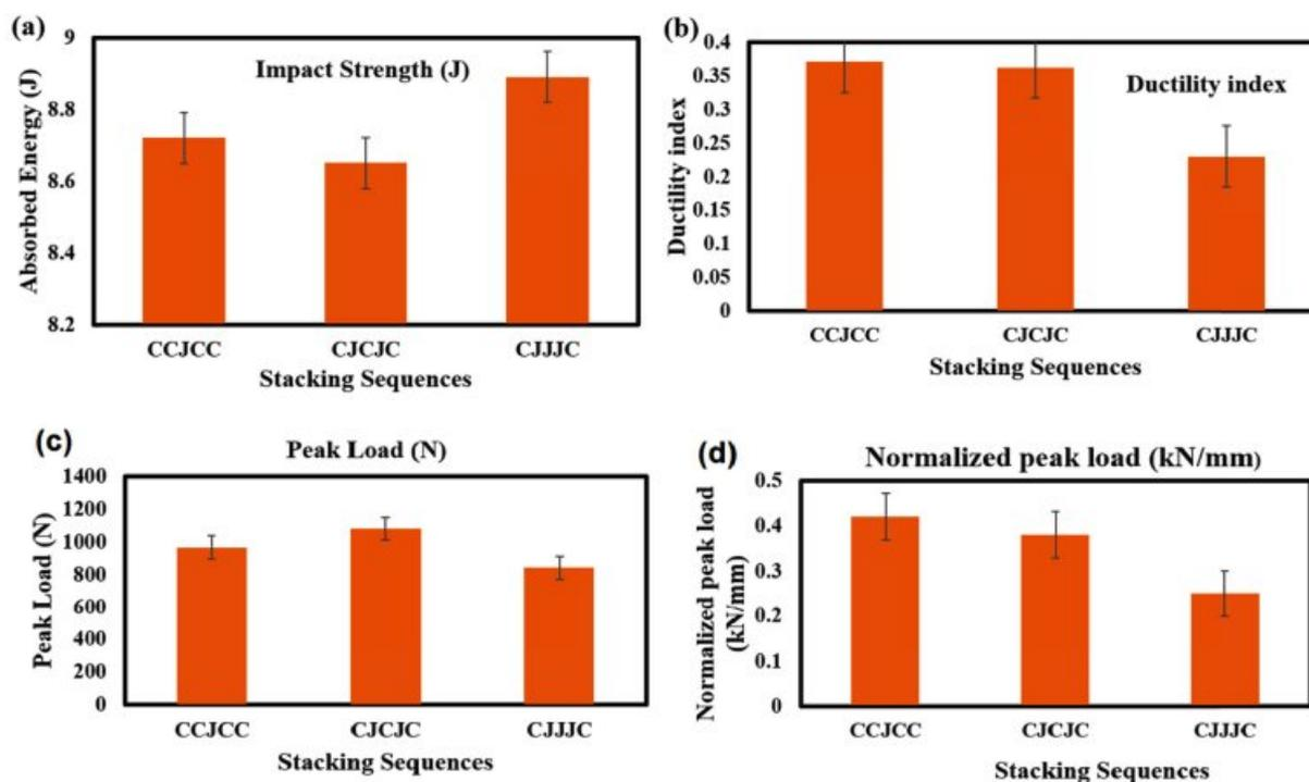
**Figure 6.** (a) Absorbed energy of laminates; (b) ductility index of laminates; (c) effect of pure carbon and its hybrids with jute on peak load at the same impact; (d) effect of pure carbon and its laminates with jute using notion of normalization.
