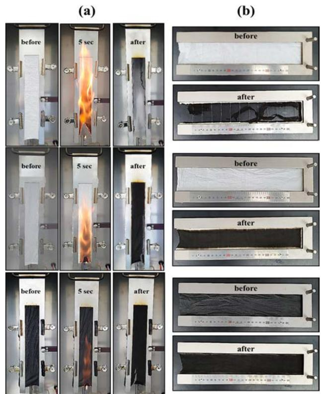
**Figure 4.** Photographs of (a) vertical; (b) horizontal flame test of untreated fabrics (top), 20 BLs of CH-C/MMT (middle) and CH-C/CNT-MMT (bottom) LbL-treated samples.
