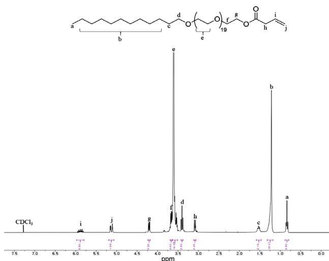
Figure 4. ^1\text{H} NMR spectrum of dodecyl-polyethyleneglycol(20) 3-butenate.
