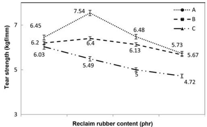
**Figure 4.** Plots of tear strength with various blend combinations of NR/BR/RR.
