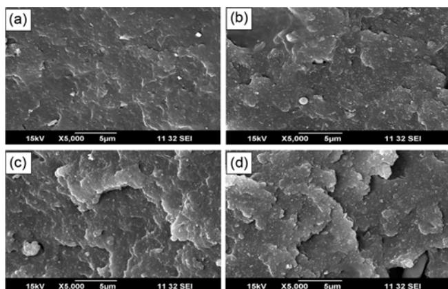
**Figure 10.** Tensile fractured surface of (a) NR/BR/RR (50/50/0); (b) NR/BR/RR (40/50/10); (c) NR/BR/RR (30/50/20); (d) NR/BR/RR (20/50/30).
