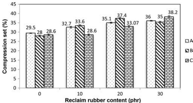
Figure 6. Plots of compression set with various blend combinations of NR/BR/RR.
