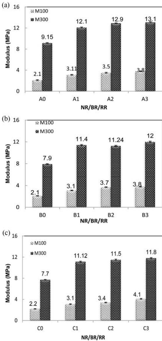
**Figure 3.** Plots of modulus of NR/BR systems with different RR loading: (a) 60/40; (b) 50/50; (c) 40/60.
