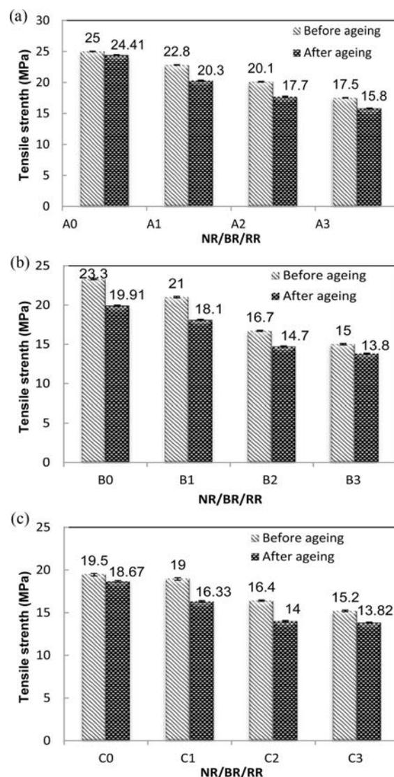
**Figure 1.** Plots of tensile strength of NR/BR systems with different RR loading: (a) 60/40; (b) 50/50; (c) 40/60.
