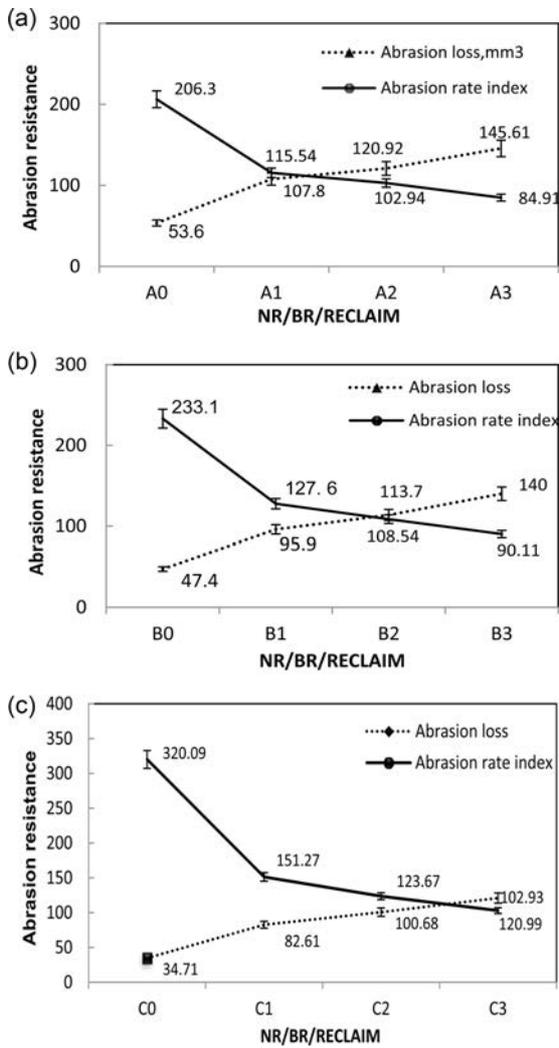
Figure 5. Plots of abrasion resistance of NR/BR systems with different RR loading: (a) 60/40; (b) 50/50; (c) 40/60.
