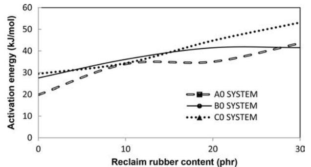
**Figure 9.** Plots of activation energy with various blend combinations of NR/BR/RR.
