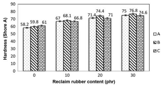
Figure 7. Hardness with various blend combinations of NR/BR/RR.
