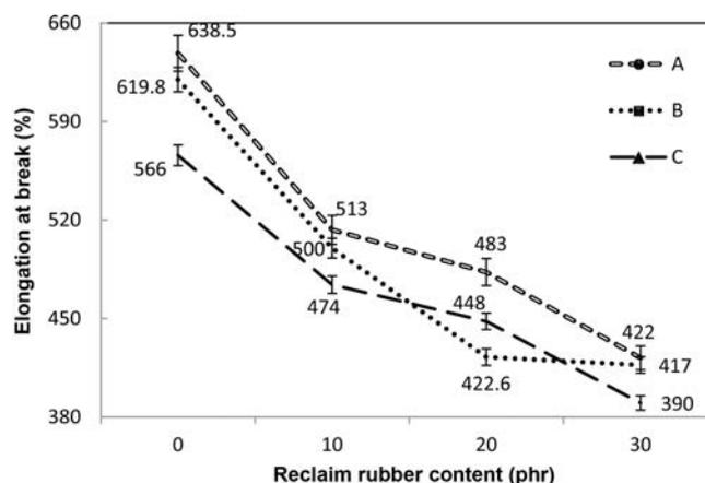
**Figure 2.** Plots of elongation at break with various blend combinations of NR/BR/RR.
