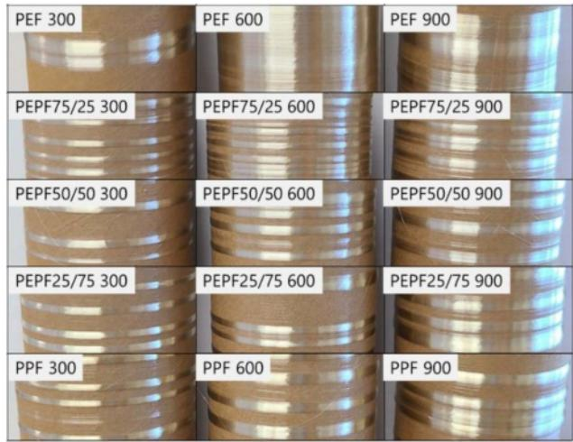
Figure 7. Melt spun copolyester fibers at winding speed of 300, 600 and 900 m/min.
