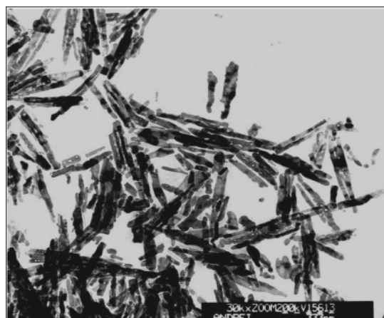
Figure 1. Cryo-TEM image of Co- \gamma -Fe 2 O 3 particle in the magnetic dispersion.
