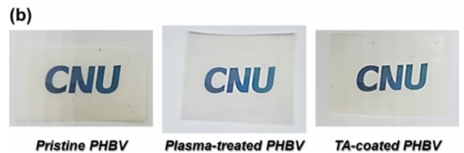
Figure 6. (a) Visible-light transmittance of the pristine, plasma-treated, and TA-coated PHBV films; (b) photographs of PHBV films on the CNU logo.
