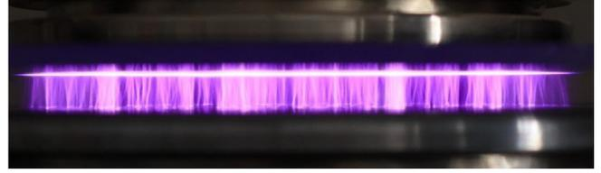
**Figure 3.** Filamentary DBD observed in the experiment.
