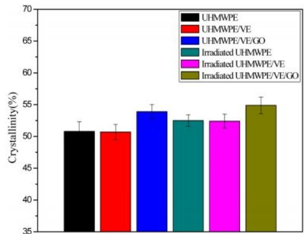
**Figure 6.** Crystallinity of different materials.
