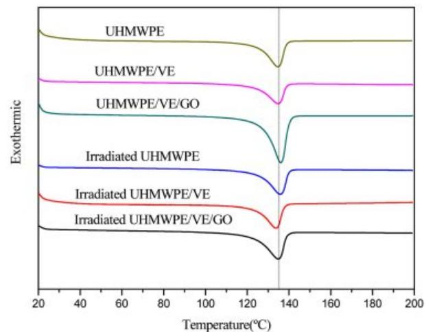
Figure 4. DSC curves of different materials.
