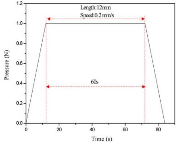
Figure 3. Diagrammatic sketch of parameters for scratch test.
