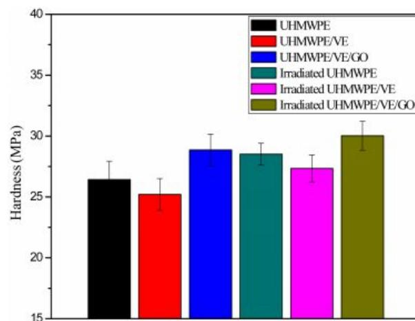
**Figure 8.** Ball indentation hardness of different materials.
