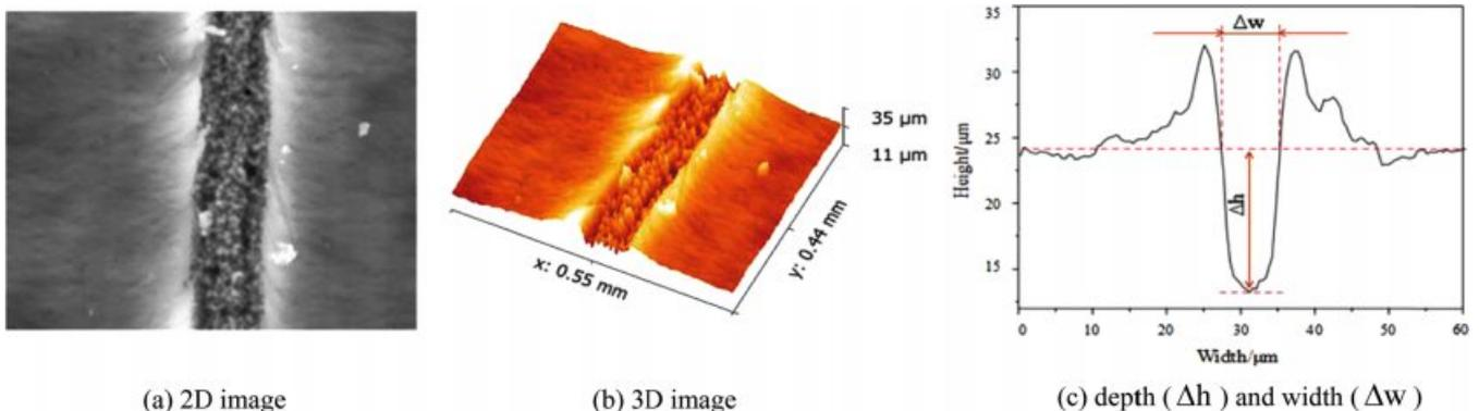
**Figure 10.** Scratch morphology of different materials.
