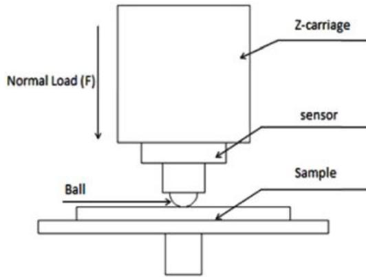
Figure 1. Diagrammatic sketch of ball indentation hardness test.
