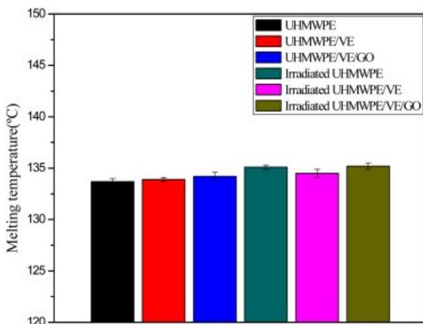
**Figure 5.** Melting temperature of different materials.
