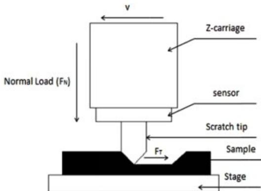
Figure 2. Diagrammatic sketch of scratch test.
