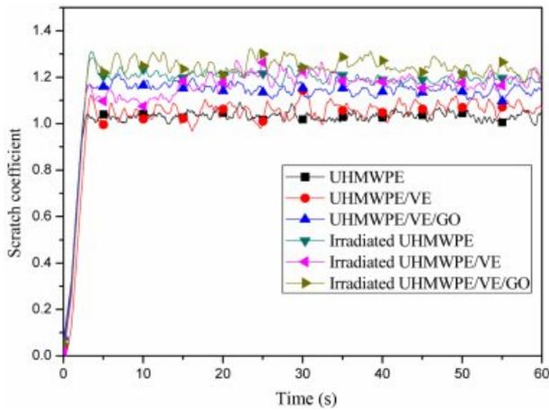
**Figure 9.** Scratch coefficient of different materials.
