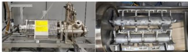
**Figure 2.** Kneader reactor (left) and twin shaft of kneader reactor (right).
