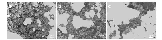
Figure S2. Smooth part of the surface SEM images of 3D printed (a) UTI, (b) UTIS1, and (c) UTIS3 is appeared as gray to calculate the area ratio of the smooth surface after Taber abrasion test.
