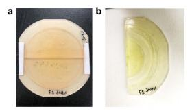
Figure S1. (a) A specimen with a shape of a disc for Taber abrasion test. Two printed semi-discs were attached to form a disc and leveled using a sandpaper. (b) A semi-disc after 10,000 cycles of Taber abrasion test. The half were separated for SEM imaging.
