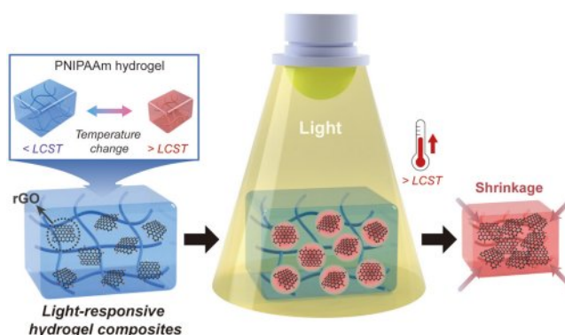
Figure 1. Schematic illustration of smart light-responsive hydrogel composites and their light-responsive swelling behavior.
