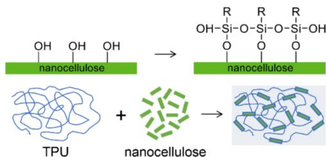
Scheme 1. Scheme of surface modification of CNC by silane coupling agents and fabrication of TPU composite. R represents -(\text{CH}_2)_3\text{NH}_2 for APTES and -(\text{CH}_2)_7\text{CH}_3 for OTES.
