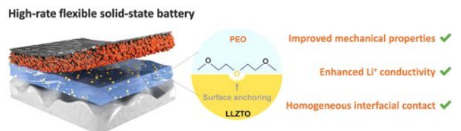
Figure 3. Proposed working mechanisms for OV-LLZTO/PEO in an all-solid-state battery. ©2023 Wiley-VCH GmbH. 78
