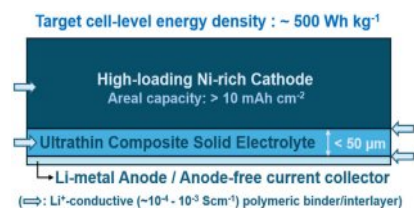
Figure 4. Conceptual cell configuration for high-energy all-solid-state batteries.
