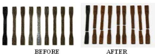
Figure 2. Tensile test specimens before and after testing.
